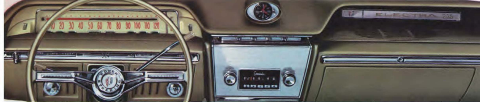
Instant instrument viewing. With Buick's Mirromagic instrument panel you see all instruments in a tilted mirror without glare or reflection.
